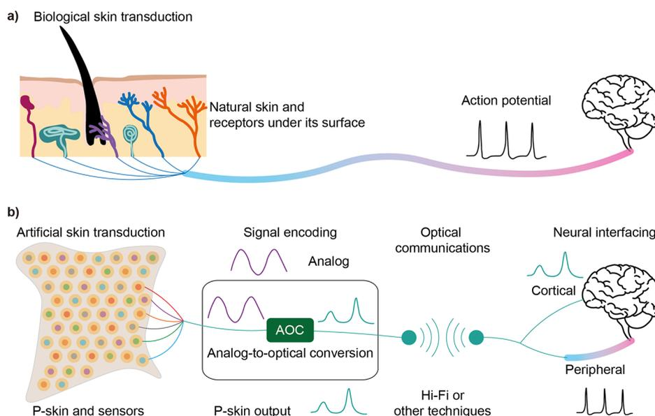
**Figure 4.** Schematics of the steps required for the transduction of sensory stimuli from (a) natural or (b) artificial receptors in the brain. Signal collection, encoding in photonic signals mimicking action potentials, photonic communications and neural interfacing are all key issues that need to be addressed to add sensing capabilities to p-skin devices.<sup>29</sup>
