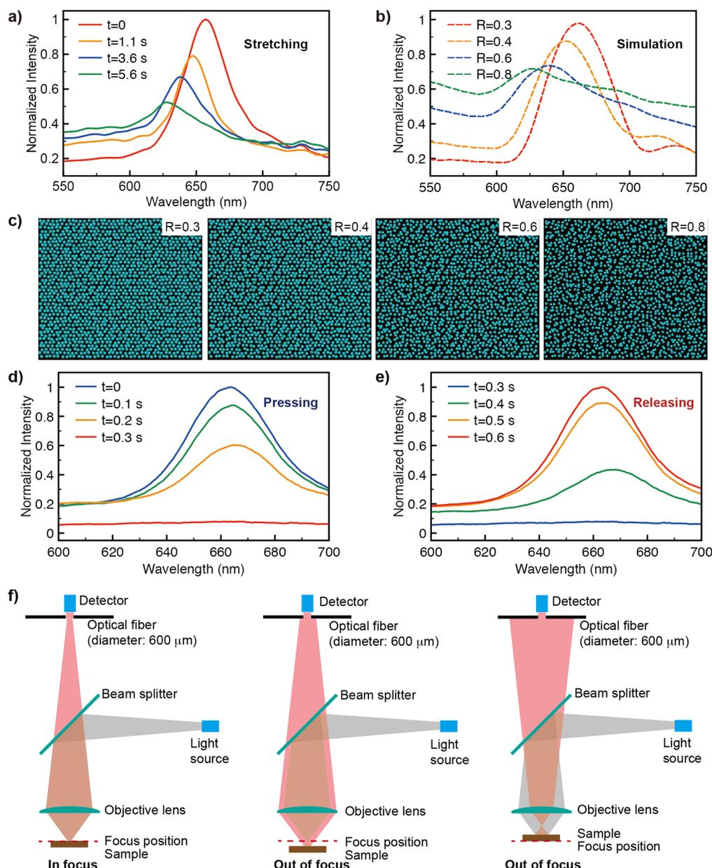
**Figure 2.** (a) The reflection spectra changed when a gel-PC sample was stretched. (b) Reflection spectra and (c) images of a simulation of PS colloidal arrays with different randomness. The reflection spectra of the gel-PC samples changed when pressure was (d) applied and (e) released at high speed. (f) Schematics of the in-focus and out-of-focus detection modes.
