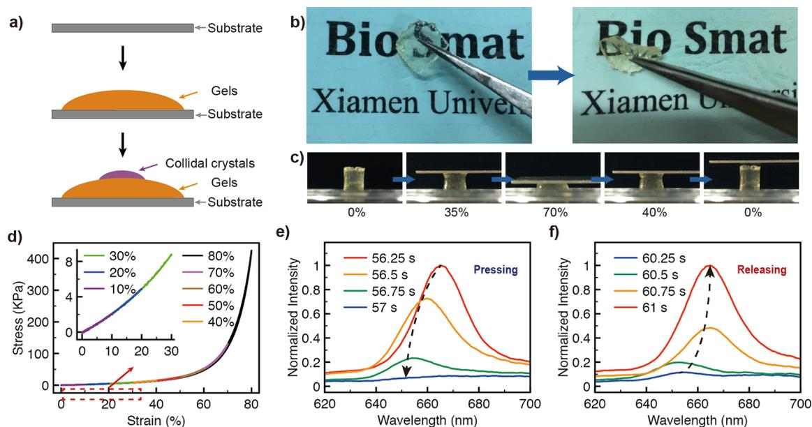
**Figure 1.** (a) Schematic of the process of sensor fabrication. (b) Photographs of the folding process of a keratin-based gel sample. (c) Photographs of a gel sample (cut into a circular cylinder 5 mm in diameter and 6 mm in height) under different pressure strains (as labeled below). (d) Mechanical properties of the keratin-based gel. (e) Reflection spectra of a gel-PC sample during the pressing process. (f) Reflection spectra of the gel-PC sample during the release process.
