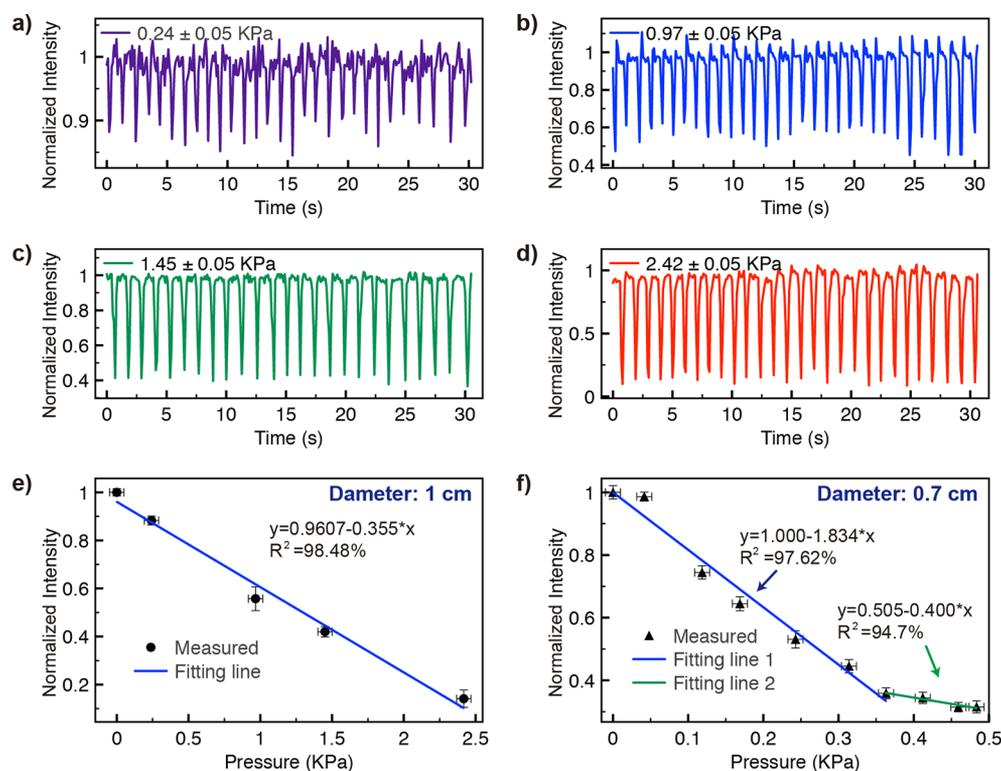
**Figure 3.** Normalized reflection intensity changes of a gel-PC sample with a diameter of 1 cm when pressed at (a)  $0.24 \pm 0.05$  kPa, (b)  $0.97 \pm 0.05$  kPa, (c)  $1.45 \pm 0.05$  kPa, (d)  $2.42 \pm 0.05$  kPa and (e) different levels (0–2.50 kPa), respectively. (f) Normalized reflection intensity changes in a gel-PC sample with a diameter of 0.7 cm when pressed at different levels (0–0.50 kPa).
